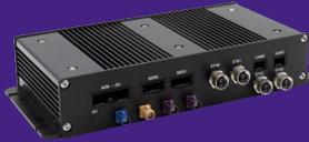
The DynaGATE 10-14 is a Road Vehicle certified, IoT Gateway for Public Transport and Road Vehicles that enables a fast transition to ITxPT in both existing and new deployments.
